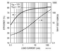
Figure 2. Efficiency and Power Loss vs Load Current
