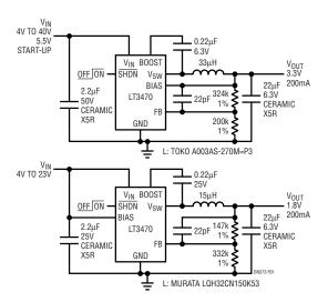
Figure 1. Typical 3.3V and 1.8V Output Applications
